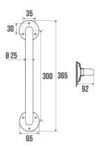
Visible fixings. Chrome and nickel-plated brass tube Ø 25 mm.
