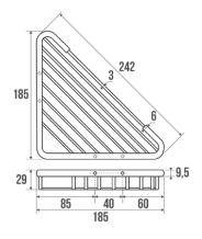
Wall-mounted. Fastening distance: 40 mm. Height: 32 mm. Wires: Ø 3 mm.
