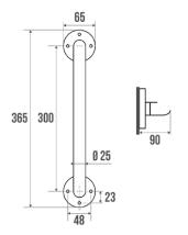
White epoxy-coated steel tube Ø 25 mm. White cover plates Ø 65 mm.
