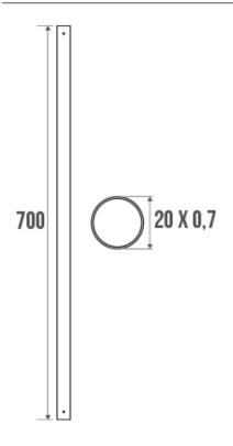
Straight tube Ø 20 x 0,7 mm for curtain rails. Can be cut to size. Perfectly suited for use in Institutions.
