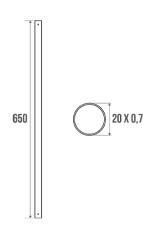
Straight tube Ø 20 x 0,7 mm for curtain rails. Can be cut to size. Perfectly suited for use in Institutions.
