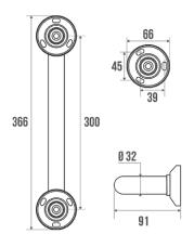
Concealed fixings. Chrome and nickel-plated brass tube Ø 32 mm. Bright chrome-plated resin flanges and cover plates.
