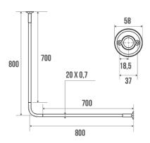
2 straight tubes Ø 20 x 0,7 mm + 2 sliding wall flanges + 1 elbow connector. Can be cut to size.
