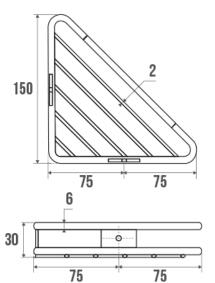
Wall-mounted. Electropolished 304 stainless steel wire Ø 6 mm and 2,5 mm.
