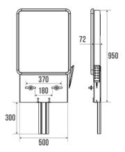
Adjustable height with electrical assistance, with remote control, up to 300 mm. In the lowest position, the adjustable wahsbasin support shall be set at 1.50 m from the ground.
