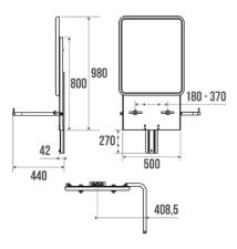
Adjustable height with a system of gas jack, up to 270 mm.
