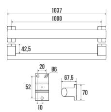
Elliptical tube in white epoxy-coated aluminium. Mat chrome-plated resin cover plates.
