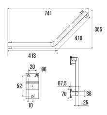
2 fixing points. Symmetrical 400 x 400 mm. Elliptical tube in white epoxy-coated aluminium. Mat chrome-plated resin cover plates.
