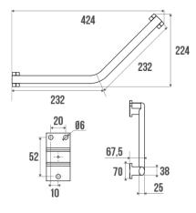
2 fixing points. Symmetrical 200 x 200 mm. Elliptical tube in white epoxy-coated aluminium. Mat chrome-plated resin cover plates.
