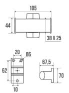
Elliptical white aluminium tube 38 x 25 mm. Mat chrome-plated resin cover plates.
