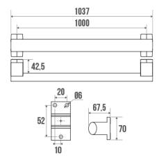
Elliptical tube in white epoxy-coated aluminium  $38 \times 25$  mm. White resin cover plates.
