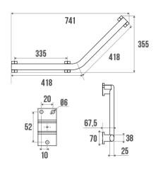
3 fixing points. Symmetrical 400 x 400 mm. Elliptical tube in white epoxy-coated aluminium. White resin cover plates. 3rd point to be fitted for right or left configuration.
