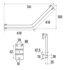
2 fixing points. Symmetrical 400 x 400 mm. Elliptical tube in white epoxy-coated aluminium.
