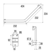
2 fixing points. Symmetrical 200 x 200 mm. Elliptical tube in white epoxy-coated aluminium. White resin cover plates.
