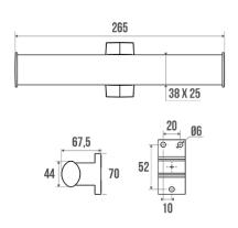
Double. Elliptical white aluminium tube 38 x 25 mm. White resin cover plates.
