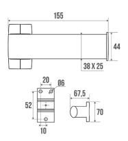
Single. Elliptical white aluminium tube 38 x 25 mm. White resin cover plates.
