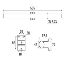
2 fixed arms. Elliptical white aluminium tube 38 x 25 mm. White resin cover plates.
