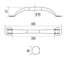
Brushed stainless steel tube Ø 25 mm. One-piece bar. Concealed fixings. Bright chrome-plated resin cover plates Ø 65 mm.
