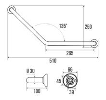
Symmetrical. Brushed 304 stainless steel tube Ø 30 mm. One-piece bar. Concealed fixings. Mat chrome-plated resin cover plates Ø 65 mm.
