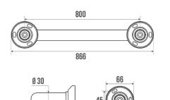
Brushed stainless steel tube Ø 30 mm. One-piece bar. Concealed fixings. Mat chrome-plated resin cover plates Ø 65 mm.
