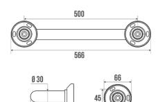
Brushed 304 stainless steel tube Ø 30 mm. One-piece bar. Concealed fixings. Mat chrome-plated resin cover plates Ø 65 mm.
