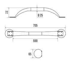
Brushed 304 stainless steel tube Ø 25 mm. One-piece bar. Concealed fixings. Mat chrome-plated resin cover plates Ø 65 mm.
