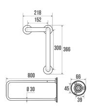
Delivered unassembled. Allows either right or left-handed configuration. White epoxy-coated aluminium tube. Blue (RAL 5002) resin cover plates.
