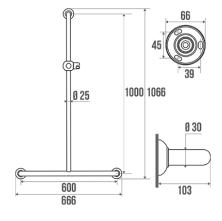
Supplied with universal clip-on shower rail slider bracket in white ABS. White epoxy-coated aluminium tube. Blue (RAL 5002) resin cover plates.
