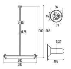
Supplied with universal clip-on shower rail slider bracket in white ABS. White epoxy-coated aluminium tube. Red (RAL 3003) resin cover plates.
