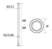
Tube Ø 20 x 0,7 mm. Supplied with flanges, screws and wall plugs.
