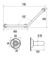
3 fixing points. Symmetrical. 135 degree angle. White epoxy-coated aluminium tube. Synthetic resin flanges.
