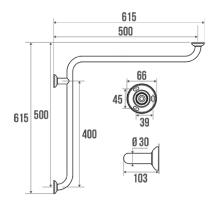
3 fixing points. Interior angle of 90 degrees. Concealed fixings. White epoxy-coated aluminium tube  $\varnothing$  30 mm. White resin flanges.
