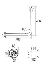
90 degree angle. Symmetrical. Concealed fixings. White epoxy-coated aluminium tube  $\varnothing$  30 mm. White resin flanges.
