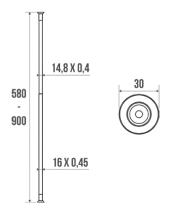
Tube Ø 16 x 0,5 mm. Supplied with flanges, screws and wall plugs. Cannot be shortened.
