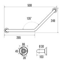
Symmetrical.#Concealed fixings. Aluminium tube Ø 30 mm. Finish: Cool Gray (Pantone 7U). Mat chrome-plated flanges and wall-fixings.
