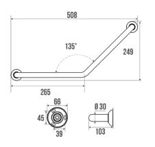
135 degree angle. Symmetrical. Concealed fixings. White epoxy-coated aluminium tube Ø 30 mm. Blue (RAL 5002) resin flanges Ø 65 mm.
