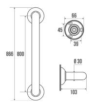
Concealed fixings. White epoxy-coated aluminium tube  $\emptyset$  30 mm. Blue (RAL 5002) resin flanges  $\emptyset$  65 mm.
