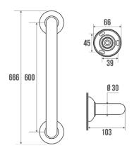
Concealed fixings. White epoxy-coated aluminium tube Ø 30 mm. Blue (RAL 5002) resin flanges Ø 65 mm.
