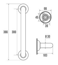
Concealed fixings. Aluminium tube Ø 30 mm. Finish: Taupe (Pantone 7591U). Mat chrome-plated flanges and wall-fixings.
