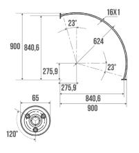
Tube Ø 16 x 1 mm. Minimum curtain width : 1400 mm 1800 mm. Cannot be shortened. 2 welded flanges.
