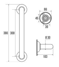
Concealed fixings. White epoxy-coated aluminium tube Ø 30 mm. White resin flanges Ø 65 mm.
