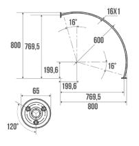
Tube Ø 16 x 1 mm. Minimum curtain width : 1400 mm 1400 mm. Cannot be shortened. 2 welded flanges.
