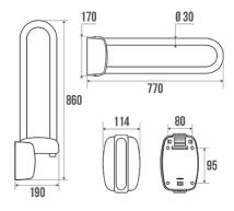
Brushed 304 stainless steel tube  $\emptyset$  30 mm. Synthetic resin flange. Vertical locking.
