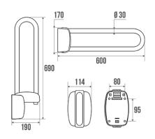
Brushed 304 stainless steel tube Ø 30 mm. Synthetic resin flange. Vertical locking.
