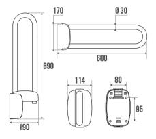
White epoxy-coated aluminium tube  $\emptyset$  30 mm. Synthetic resin flange. Vertical locking.
