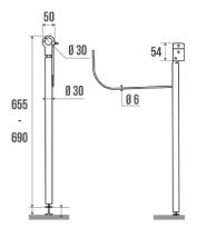
Use of the prop is recommended when the fixing wall is not strong. Possibility to fix the toilet roll holder ref. 048820 to the hinged bar.
