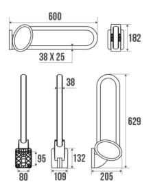
Concealed fixings. Elliptical tube 38 x 25 mm in anthracite grey epoxy-coated aluminium. Wall flange, joint and side plates in Bright chrome-plated synthetic resin.
