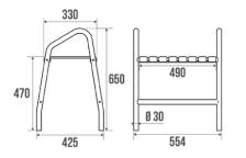
Taupe (Pantone 7591U) polypropylene seat. Grey epoxy-coated aluminium tube. 4 non-slip plastic foot caps. Enables users to sit down safely and comfortably while showering.
