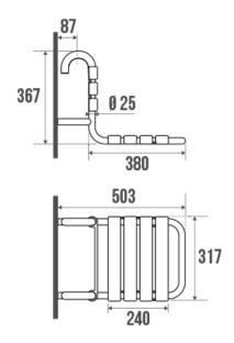
To hang on grab bars Ø 30 mm, Ø 32 mm (aluminium, stainless steel, brass) or Ø 33 mm (polyalu), length 400 to 800 mm (grab bar not included). White polypropylene slats.
