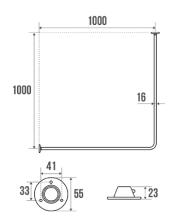
White epoxy-coated steel tube Ø 16 x 0,5 mm. Can be cut to size. 2 sliding wall flanges made of white ABS.
